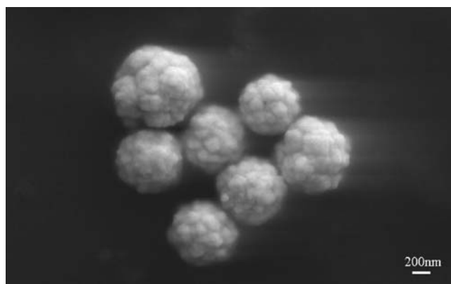
Fig. 6. SEM image of the W/O/O particles with encapsulated rhodamine and a silver cage on the exterior of the particle.
